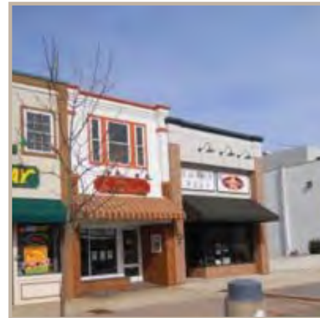
New buildings should be within a few feet in height of its neighboring structures, with similar heights in cornices, window heads and sills, and first floor elevation above the ground. New construction should respect established rhythms of the streetscape.
