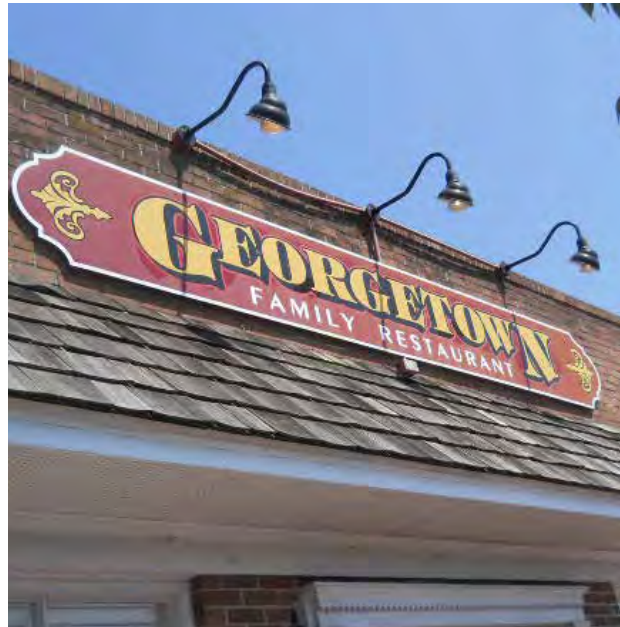
A small, well-crafted sign from Georgetown DE, fits within the traditional sign band on this one story building and has goose neck lamps that illuminate the sign at night.
