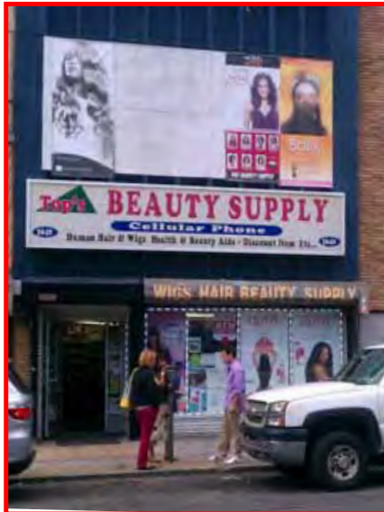
Internally lit signs are prohibited on the exterior of buildings in the historic district because they create a plastic feel.
