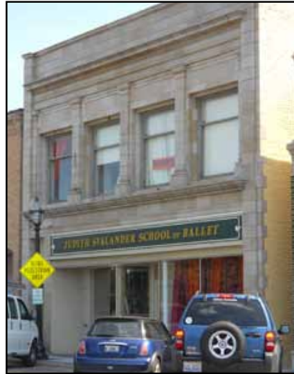
Generally, the appropriate zone for signage is above the storefront windows and below the sills of the second floor windows.
