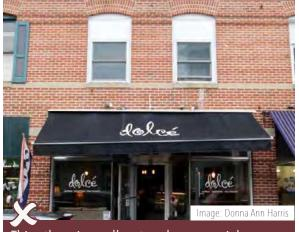
This otherwise well restored commercial building in Milford, DE has replacement windows on the upper story that do not fill the window opening. It is not recommended to reduce the upper story window size to an area smaller than the original in Haddon Heights.
